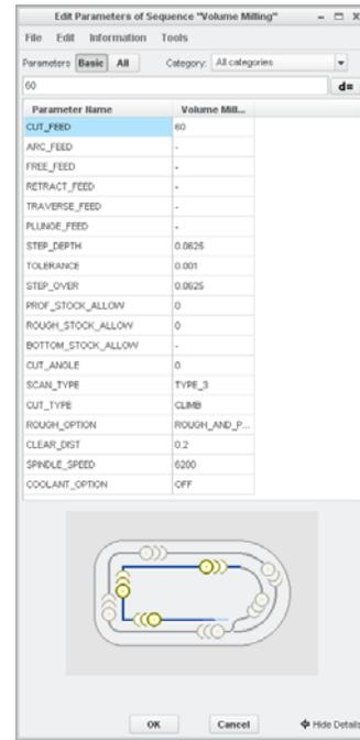
**Step 7:** Enter the manufacturing parameters shown above.
